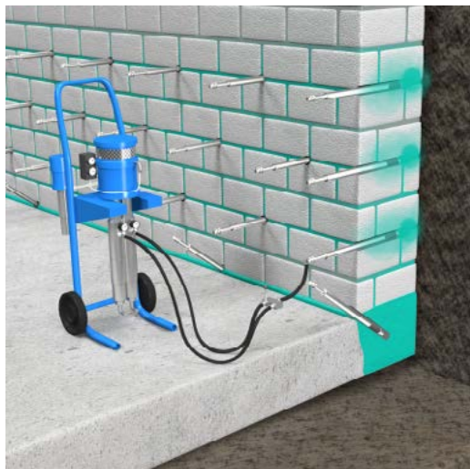
STRUCTURAL INJECTION Sealing the old wall by injecting acrylic resin.
